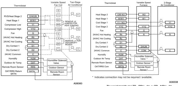
Edge Thermidistat Models TP-PRH-01 & TP-NRH-01 w/ Fan Coil & 2-Stage Air Conditioner
